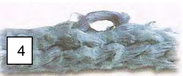
> Image 4 Strand reduced by 25% abrasion
