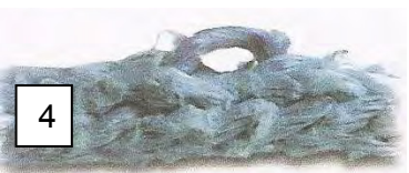
> Image 4 Strand reduced by 25% abrasion
