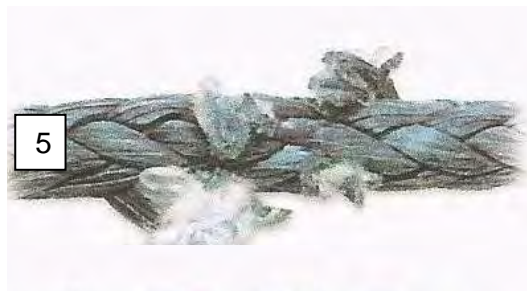
> Image 5 Rope displays two adjacent cut strands.
