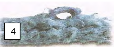
> Image 4 Strand reduced by 25% abrasion
