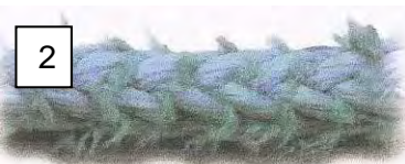
> Image 2 Rope displaying 25% reduction from abrasion
