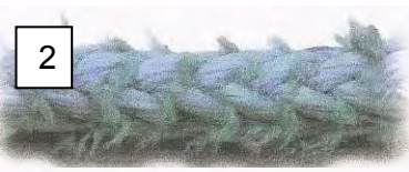
> Image 2 Rope displaying 25% reduction from abrasion
