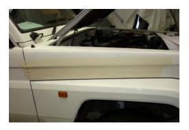
4 Tape template to mudguard making sure it is lined up with top of mudguard (bonnet opening) and rear of mudguard (door opening). Using a felt tipped pen, mark all holes through template onto mudguard. Remove template.
