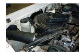
16. Check all hose connections for potential leaks and seal as required.
