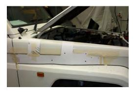
5. For snorkel outlet, using an 89mm hole saw cut two semi circles as shown. Mark a line between top and bottom of the semi circles and cut along lines using an air hack saw.
