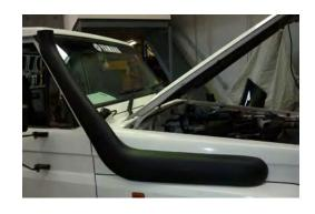
13. Insert smaller diameter end of rubber intake hose through inner guard and attach to snorkel and secure with hose clamp provided.
