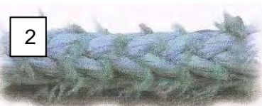
> Image 2 Rope displaying 25% reduction from abrasion
